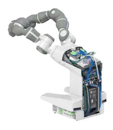
Embedded controller based on IRC5
